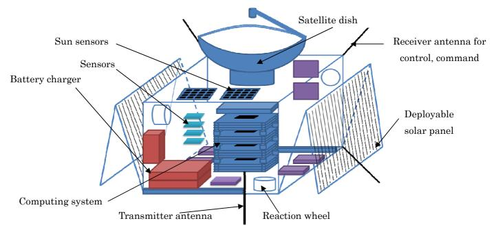
Figure 1- Illustration the Radio Telescope Nano-satellite
