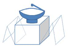
Side View - Partially deployed solar panels
